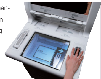
ATM equipped with a finger vein authentication system
