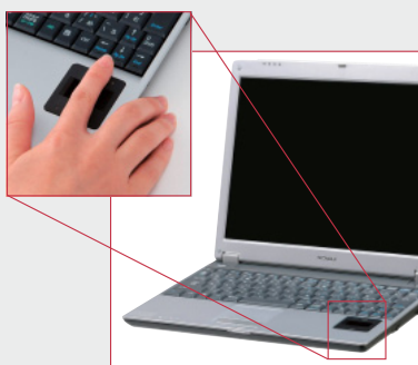
This security PC has an in-built finger vein authentication system, but no internal HDD
