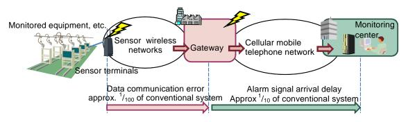
Wireless network remote monitoring system configuration
