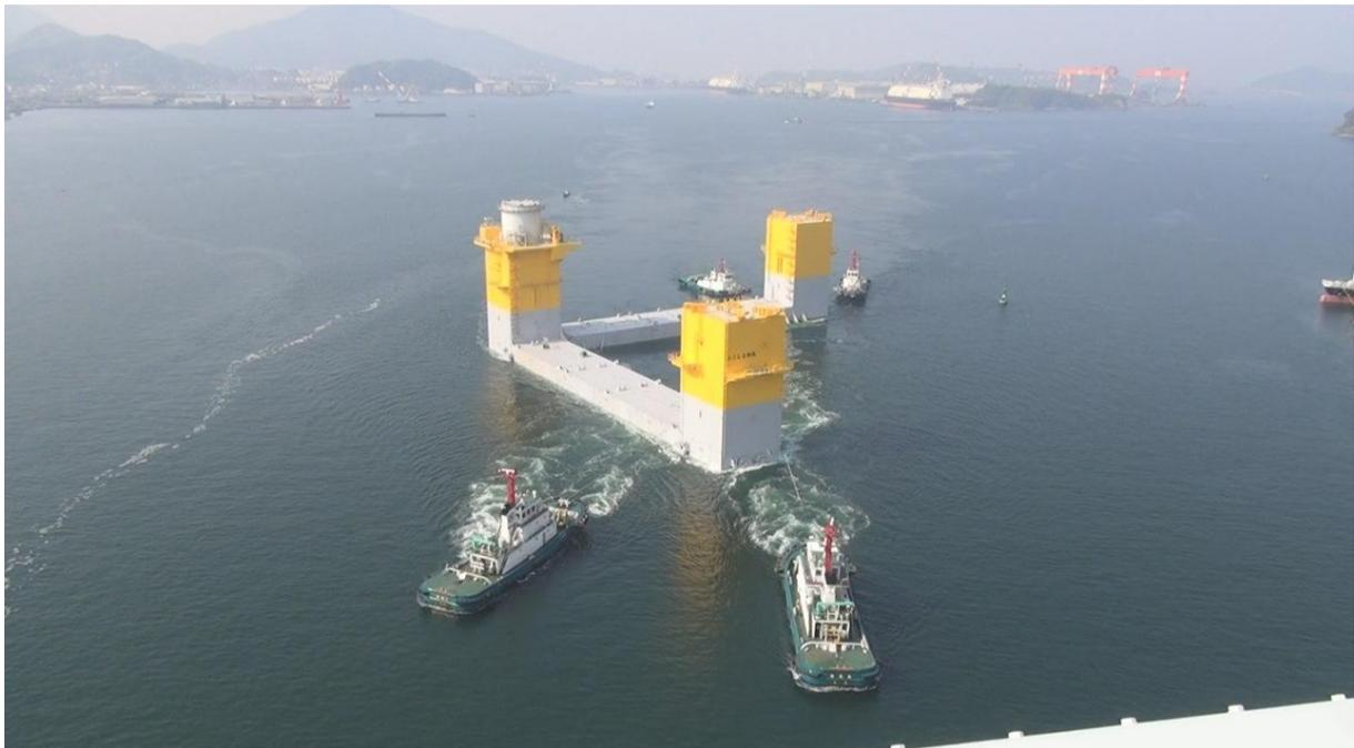
**Towing the three-column semi-sub at Nagasaki port**
