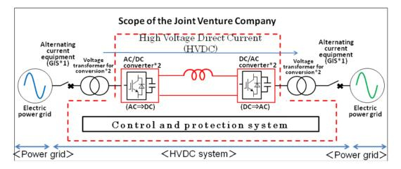
HVDC systems are used to transfer power between two electric power grids. The system converts the supply side power from AC to DC and transmits the power in DC form. On the receiving side, the power is converted back into AC again to be used.
