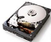
1-terabyte 3.5-inch hard disk drive by Hitachi Global Storage Technologies
