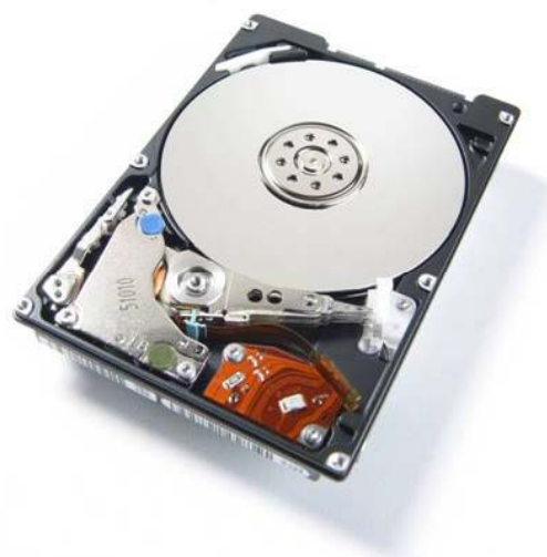
Figure 3.2 Travelstar 5K160: 160 GB 2.5" Hard Disk Drive using PMR Technology
