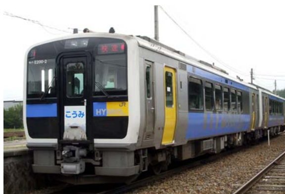
Fig. 2.3 JR East's Series E200 Motor DEMU incorporating hybrid propulsion system
