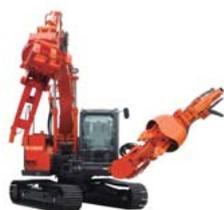
Hitachi Construction Machinery's double-arm working machine
