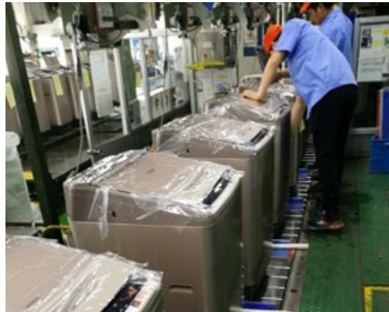
An automatic washing machine acceptance test.
