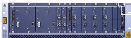
10 Gbit/s transponder (4-slot width) GbE / FC transponder (1-slot width) STM-1/OC-3, STM-4/OC-12, STM-16/OC-48 (2-slot width) Wavelength division multiplexer (1-slot width)
