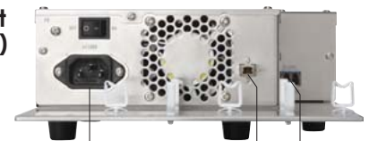
Power supply WDM interface Client interface
