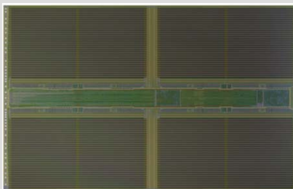
4 Gbit AG-AND Flash Memory with high-speed multilevel programming circuit technology
