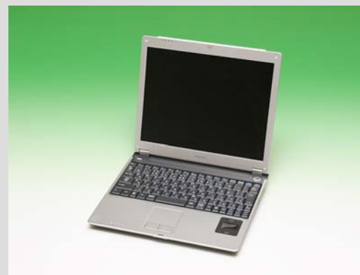
Prototype note-PC with embedded finger vein authentication unit
