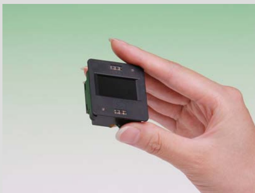
Compact finger vein authentication unit Volume 19ml [39mm(d) × 34mm(w) × 15mm(h)]
