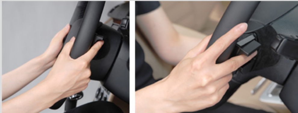
Finger vein authentication technology embedded on the steering wheel
