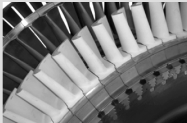
Bucket fitted on a H25 gas turbine
