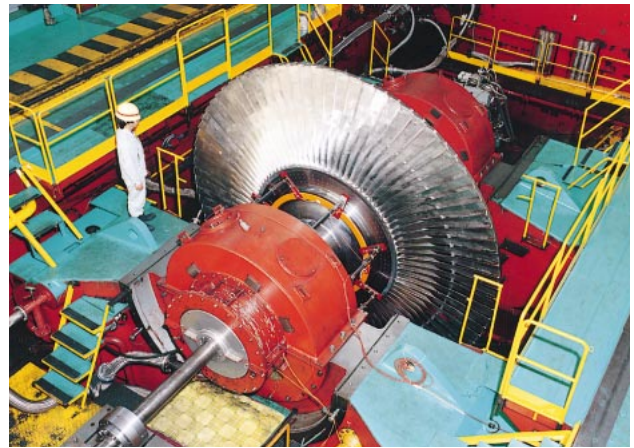
Fig. 6—Rotational Vibration Test of New 43-inch Blade with Full-scale Model Rotor.
