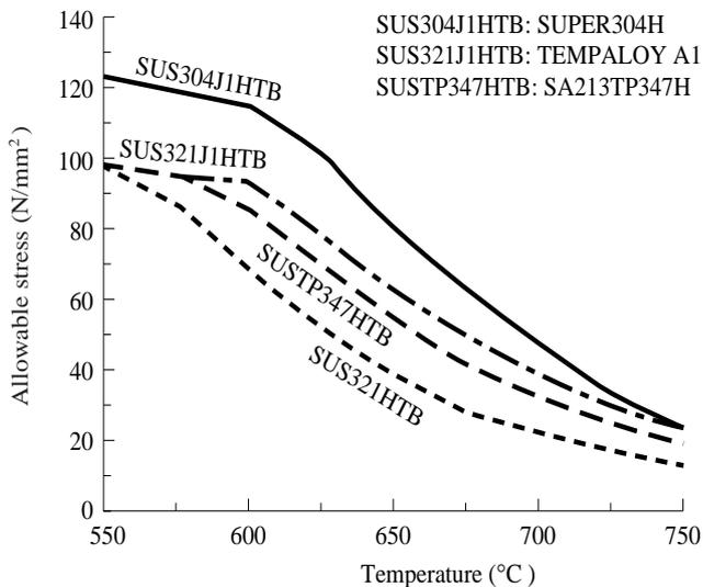
Fig. 4—Allowable Stress Data of High-Strength Austenitic Steels.
