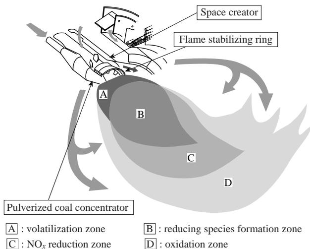
Fig. 5—Flame Structure of Hitachi-NR2 Burners. Pulverized coal concentrator and space creator accelerate high-temperature in-flame NO<sub>x</sub> reduction.
