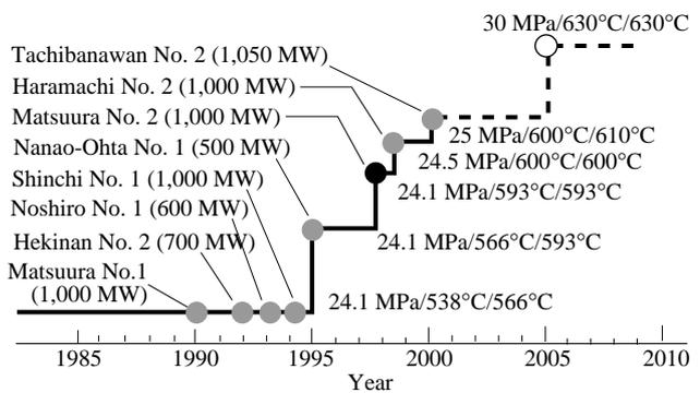
Fig. 2—Improvements in Steam Conditions of Babcock-Hitachi Boilers.
