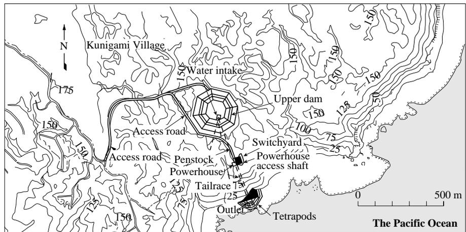
Fig. 2—Plan View of Seawater Pumped-storage Power Plant. The octagon-shaped upper dam is located 500 m away from seashore at the elevation of 150 m.
