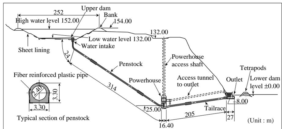
Fig. 3—Sectional View of Waterways. The underground powerhouse is situated 150 m below ground level.
