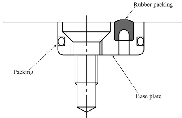
Fig. 5—Structure of Wicket Gate Seal Packing.
