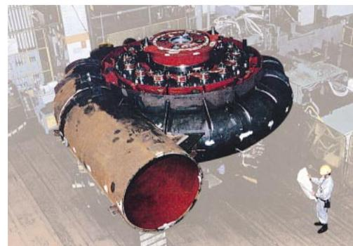
Fig. 4—Sectional View of Pump Turbine and Appearance of Pump Turbine During Shop Assembly. The runner can be taken out from below, leaving pump turbine main parts and generator motor as they are, for easy maintenance work.
