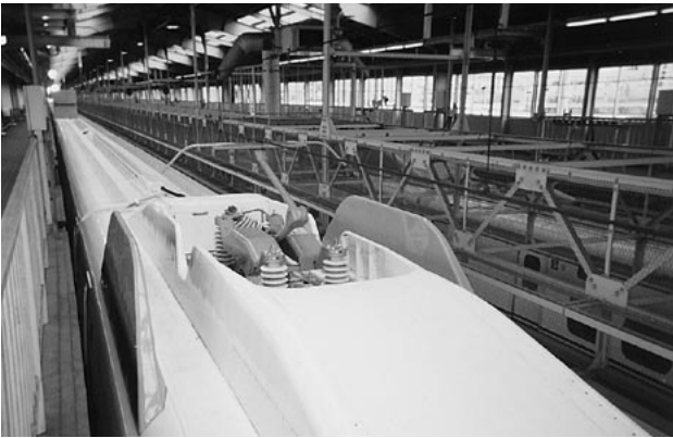
Fig. 5— Insulator Cover. The insulator cover has a wineglass shape. One pantograph is installed for every two cars, and both these points help to reduce noise outside the car.
