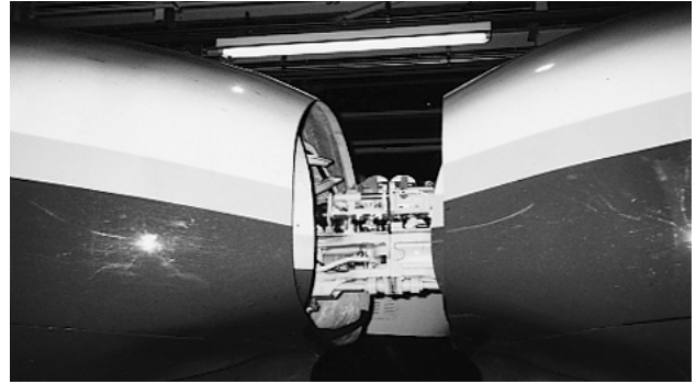
Fig. 8— Separation and Coupling Equipment. The separation and coupling equipment which couples the E4 series and the E2 series to adjust transportation capacity is installed.
