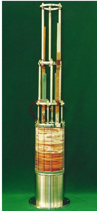
Fig. 5— Photograph of 20-Stack Double Pancake Magnet. Outer diameter is 158 mm, inner diameter is 64 mm, height is 220 mm. Tapes totaling 1 km were used for winding. Max. field 18 T at 18-T backup magnetic field.
