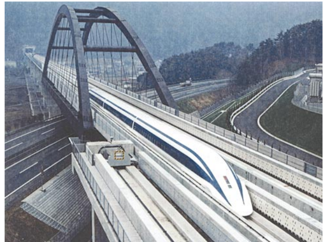
Fig. 3—External View of the Yamanashi Maglev Vehicle. Achieved a world record of 552 km/h in April 1999. (Photo by Railway Technical Research Institute)
