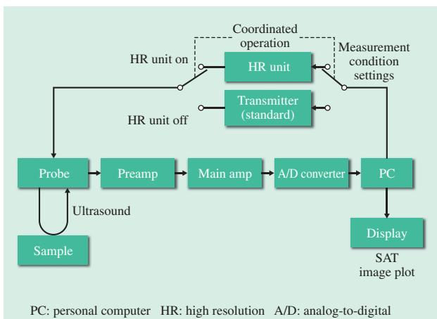
*Fig. 3—Block Diagram When Optional HR Unit is Connected. The HR unit has a function that narrows the bandwidth of the frequency components of the ultrasound emitted by the probe and shifts its frequency higher.*
