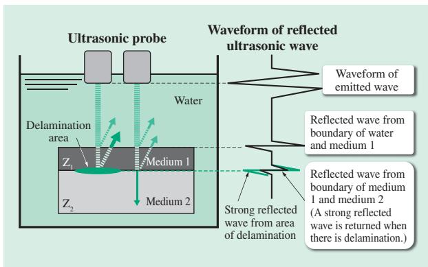
*Fig. 2—Principles of Defect Detection Using Ultrasound.
