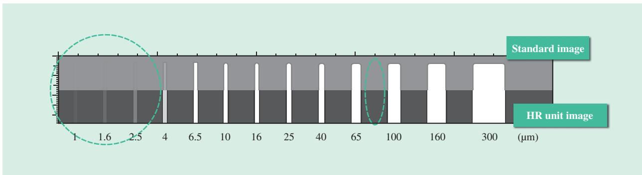
Fig. 6—Improved Detectability Using the HR Unit.
