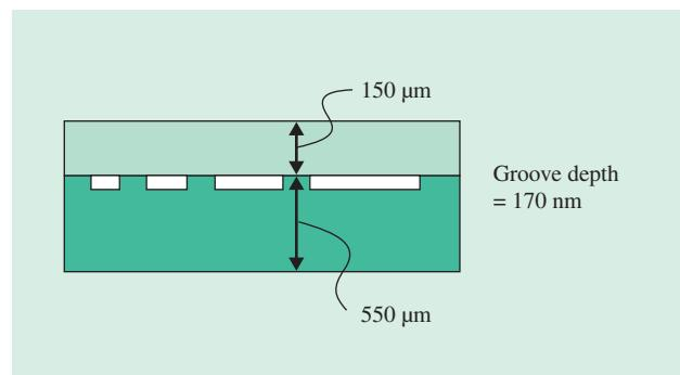
*Fig. 5—Cross-sectional Structure of Bonded Silicon Dummy Sample.*
