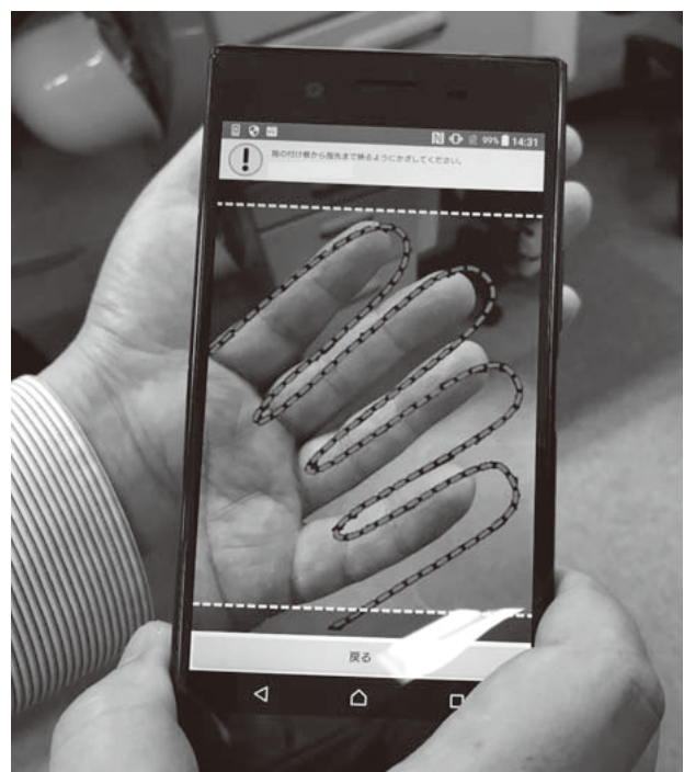
Figure 3 — Prototype of Visible-light Camera-based Finger Vein Authentication Software
