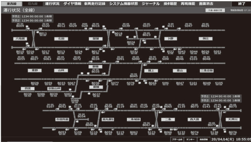
Figure 4— Example of a Traffic Status Screen The human machine interface (HMI) of the dedicated terminals is integrated with the traffic management console and the training system. The screens that can be displayed and utilized are restricted for each dedicated terminal.
