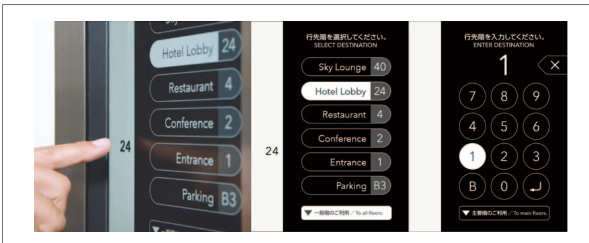
3 Touchless operation panel (prototype) demo operation and display screen
