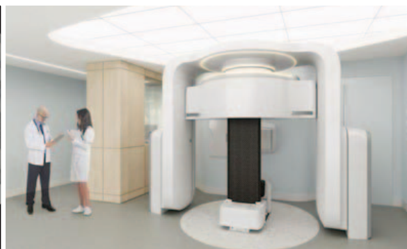
7 Image of the proton beam therapy system (left figure) equipped with a rotating gantry (center) and the UPPS (right) and the UPPS from Leo Cancer Care (right figure)
