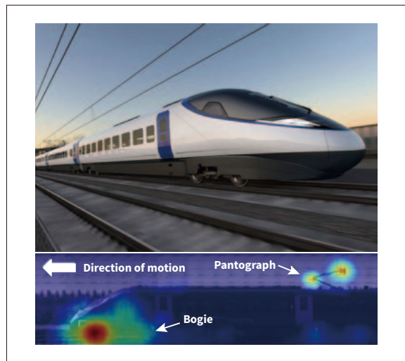
8 Artist's impression of HS rolling stock (top) and visualization of noise (bottom)
