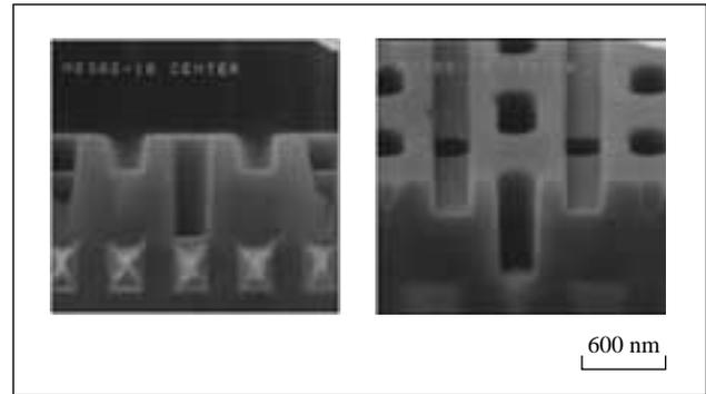
Fig. 7—Examples of SiOF Film Damascene Etching Processing. In UHF-ECR etchers, processes for etching damascene masks, holes, trenches, and bottom films can be easily implemented by controlling the gap and antenna bias.
