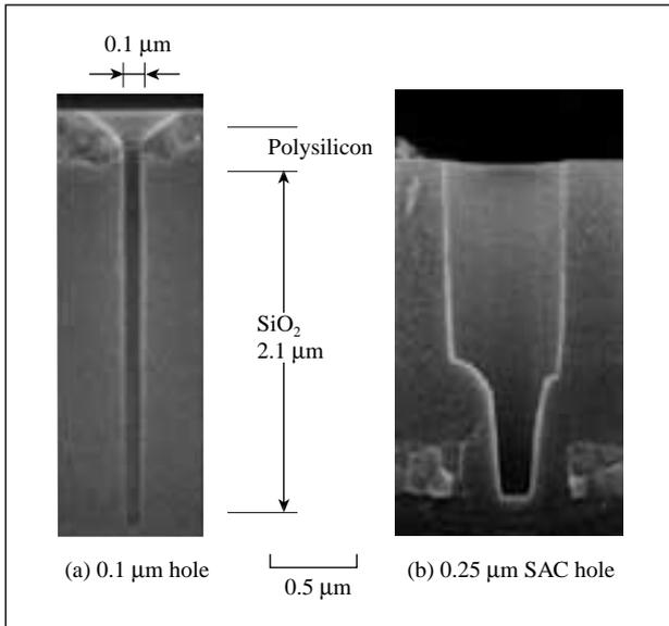
Fig. 6—Examples of Hole Etching Processing. Good hole opening and high mask selectivity are obtained by controlling  $CF_2/F$  radicals ratio and  $CF_2$  to ion ratio. In self-aligned contact (SAC) processes, good vertical profile and high SiN shoulder selectivity are obtained.
