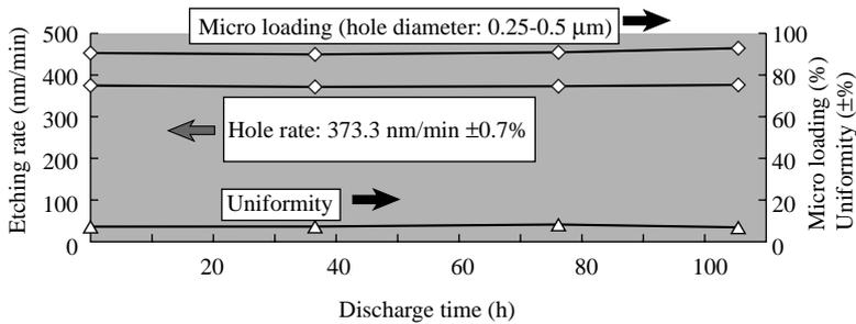
Fig. 9—Continuous Processing Stability Test Results.
