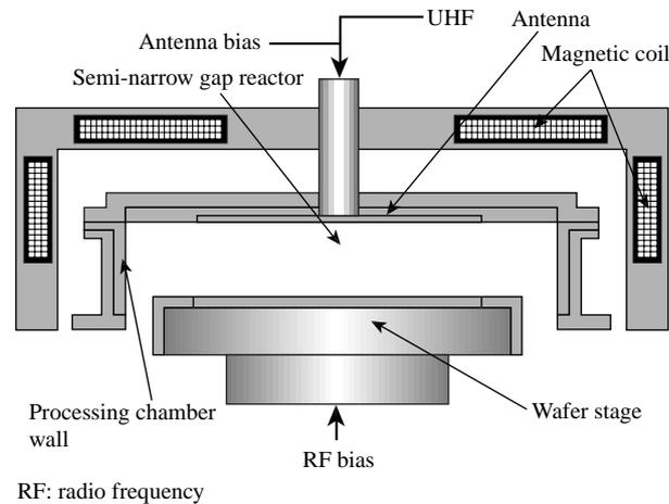
*Fig. 2—Schematic Representation of Insulating Layer UHF-ECR Etching Chamber.*
