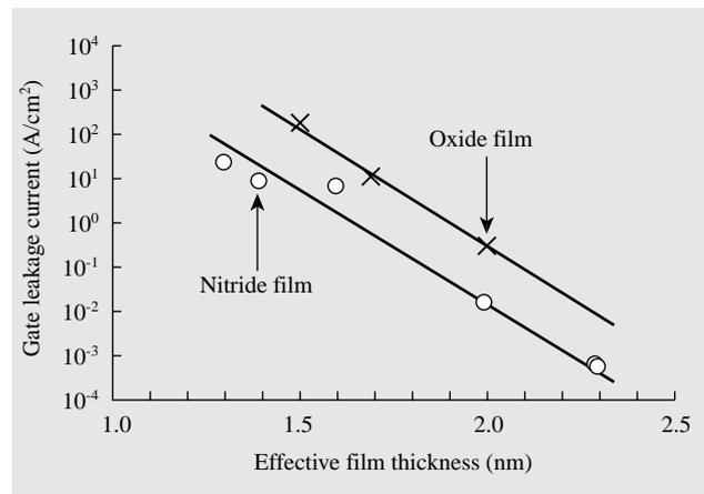
Fig. 2— Gate-Leakage Currents Through Oxide and Nitride Films.
