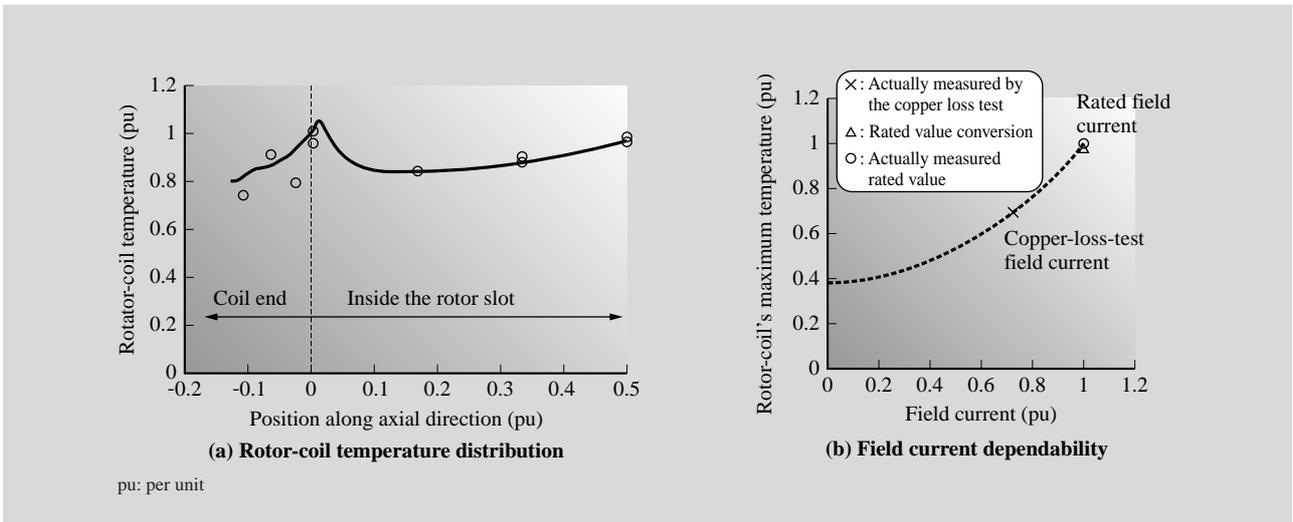
Fig. 6—Rotor-coil Temperature Distribution. A rated field current test evaluated the temperature under field operation; it was determined that the maximum temperature in the coil end was within the standard.
