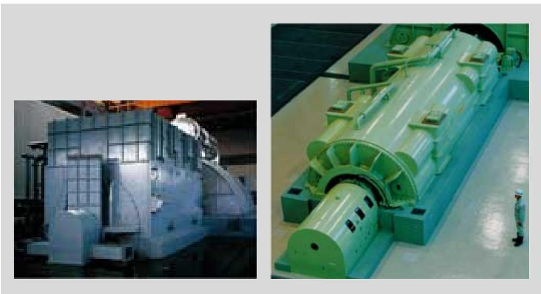
*Fig. 1—Air-cooled Generator (left) and Hydrogen and Water-cooled Generator (right). The high-reliability evaluation technology has wide applications—from 250-MVA class large-capacity air-cooled generator (left) to 800-MVA class large-capacity hydrogen and water-cooled generator (right).*
