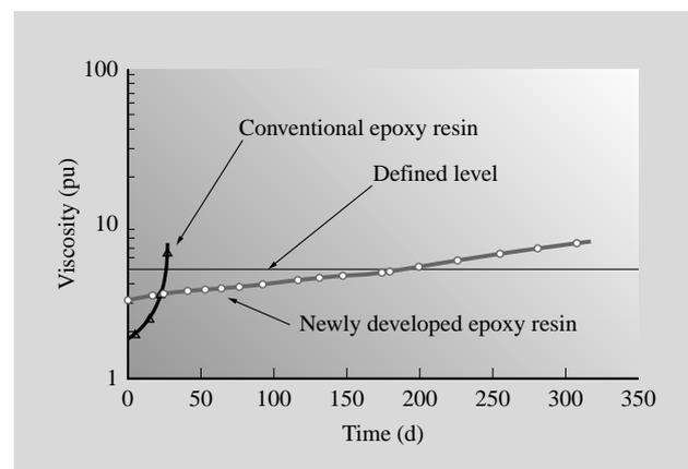
Fig. 8—Changes in Resin Viscosity with Time.
