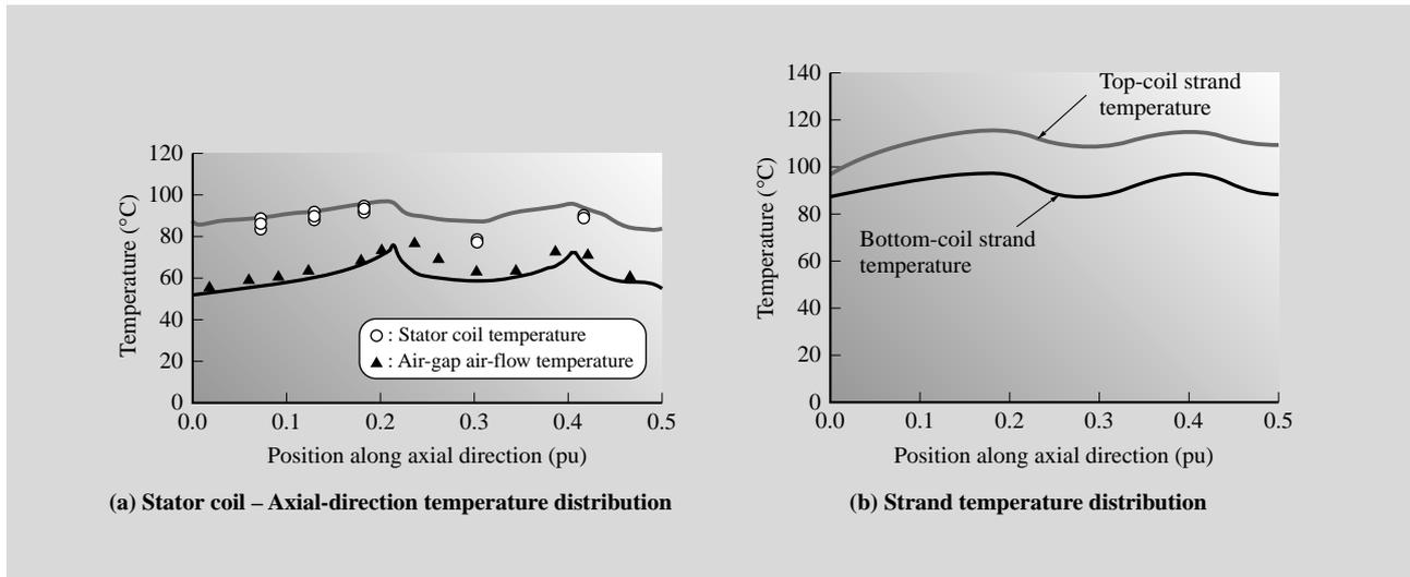
Fig. 7—Stator-coil Temperature Distribution.
