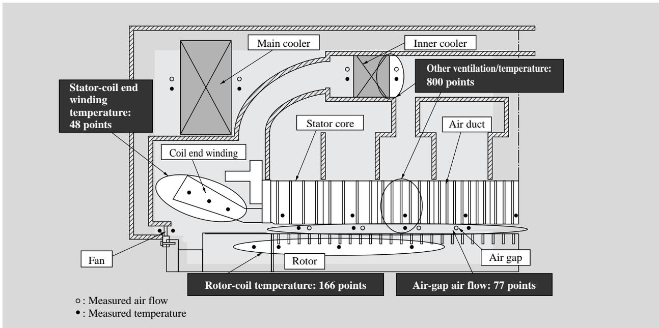
Fig. 2—Main Measuring Points of Generator.
