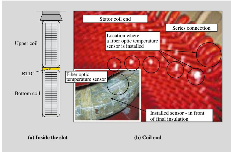
Fig. 5—Stator-coil Temperature Measurement. The temperature inside the slot was measured. An RTD was embedded between top and bottom coils; a fiber optic temperature sensor was inserted in the coil end unit.
