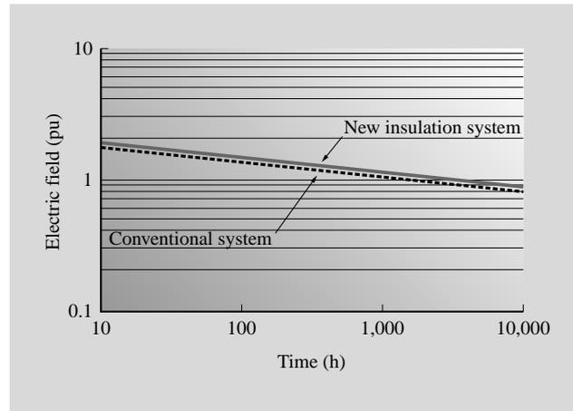
Fig. 10—Voltage-endurance Test.
