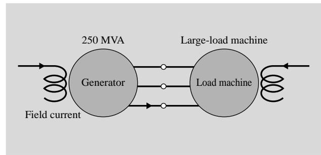
Fig. 4—Rated Field Current Test – Circuit Diagram.
