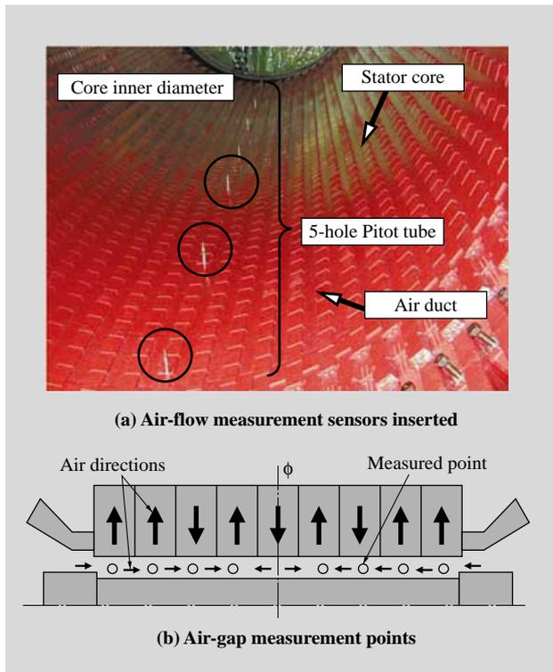
Fig. 3—Air-gap Air-flow Measurement.
