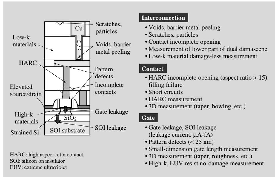
short time frame, then working to enhance the device yield (including quality and reliability) as quickly as possible after the fab is up and running. A number of technologies are critically important in this process: technologies for in-line assessment of device patterns based on device design data, technologies for verifying faults, and technologies for evaluating the electrical characteristics of devices and for verifying the completed level of the final fine structure.
