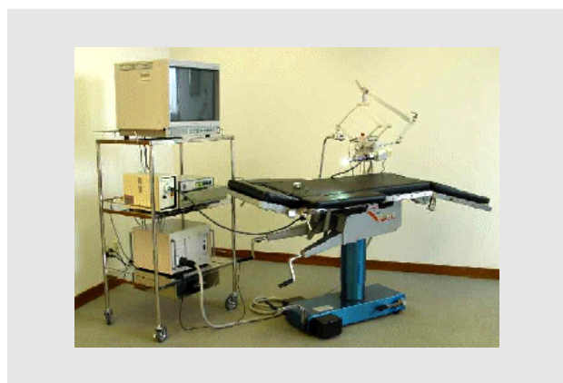
Fig. 9—Overview of Endoscopic Manipulator System. The manipulator portion is attached near the center of the bed. The main unit and other peripheral modules are on the left in the photo.
