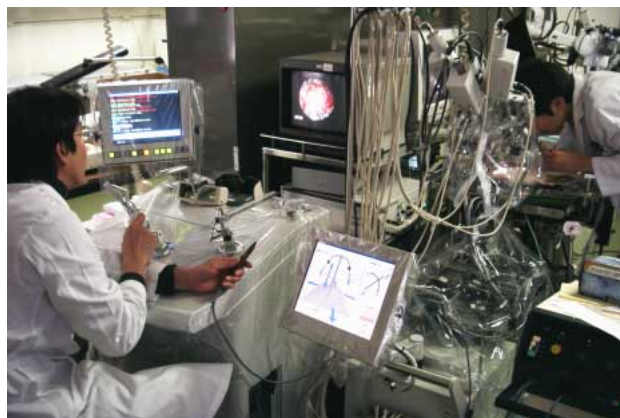
Fig. 8—A Clinician Tests the System's Capabilities. Clinical trials revealed that washing and sterilization procedures presented particular problems for surgical robotics, an issue that has to be assessed from a medical standpoint for the system as a whole.
