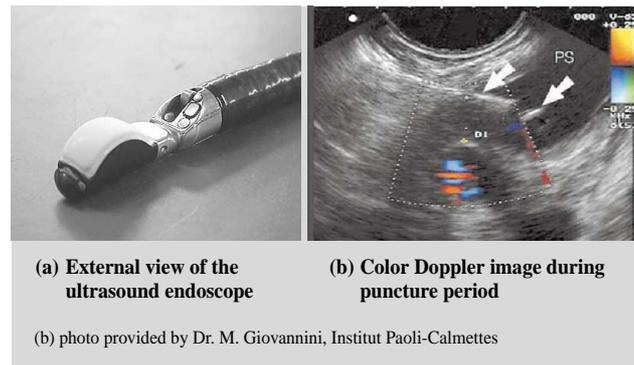
Fig. 9—Ultrasound Endoscope and Image of Puncture. In (b), the puncture needle is indicated by the arrow.
