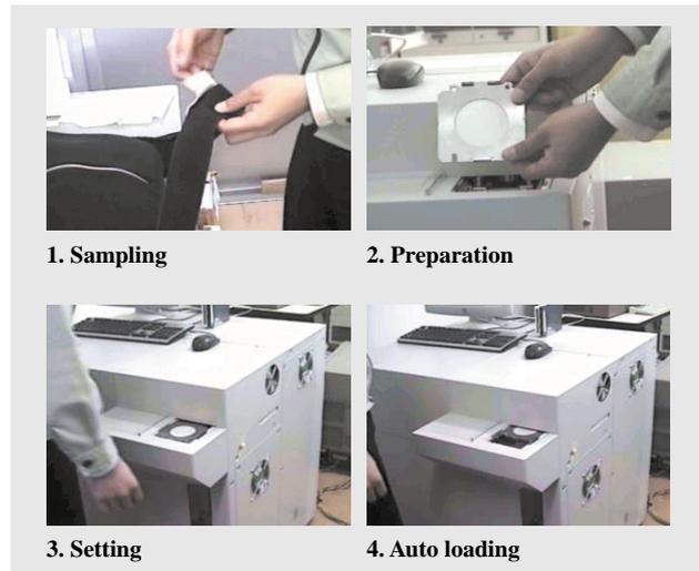
Fig. 4—Operation Procedure for Drug-trace Detection. Once the wipe material is set in the predetermined place, measurement is performed automatically.
