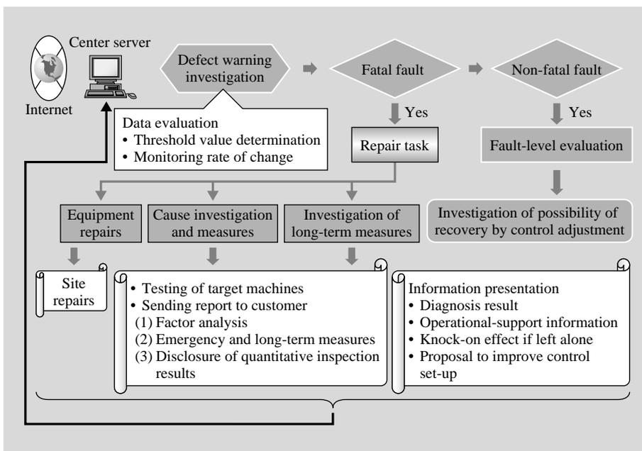
Fig. 6—Process Flow of Monitoring and Diagnosis. Based on plant information obtained by monitoring devices, the system diagnoses soundness and abnormalities, and when it detects warning signs, it assists cause investigation and fault restoration.
