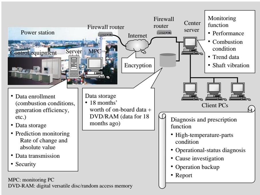
Fig. 5—Overview of Remote-monitoring System. Analog and digital data from control devices are accumulated at the Hitachi Monitoring Center via the Internet and used to monitor and diagnose plant soundness and abnormalities.
