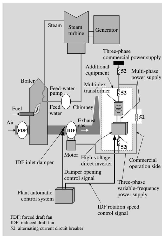
Fig. 3—System Configuration.
