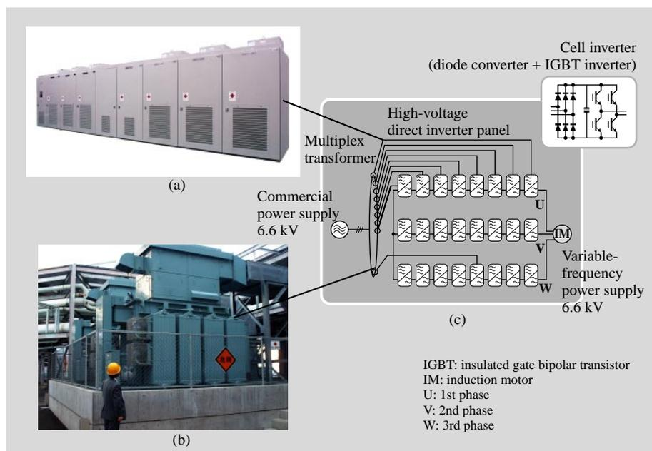
This motivated Electric Power Development Co., Ltd. and Hitachi, Ltd. to jointly develop a high-voltage high-capacity direct inverter that can also be applied to large auxiliary motors (see Fig. 2). The new inverter was applied to Electric Power Development Co., Ltd.'s Takehara Thermal Power Station No. 3 and excellent results have been obtained in the trial operation.
