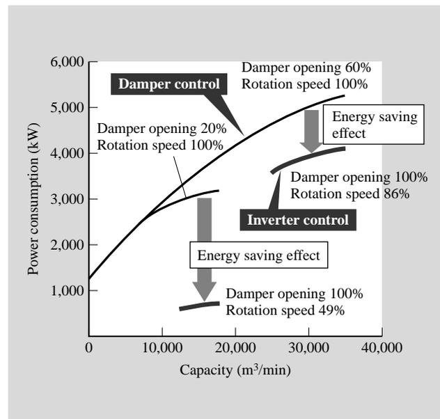
Fig. 1—Power Consumption Reduction Effect with Inverter Control.
