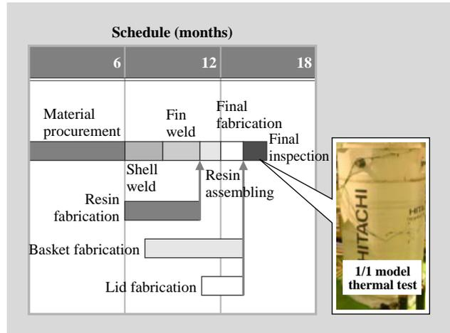
Fig. 7—Fabrication Schedule of 1/1 Scale Model.
