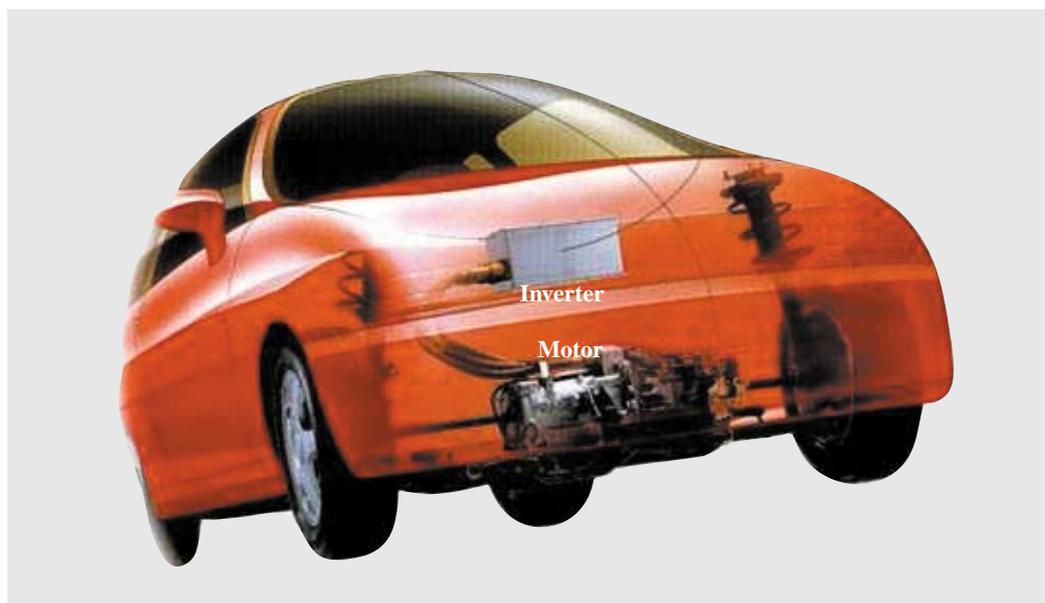
Fig. 2—Reduction of Size and Weight of Motor for HEVs. Progress in reducing the size and weight of motors for HEVs, and technologies enabling the downsizing are shown. We are now making headway in the development of a 6th-generation motor.
