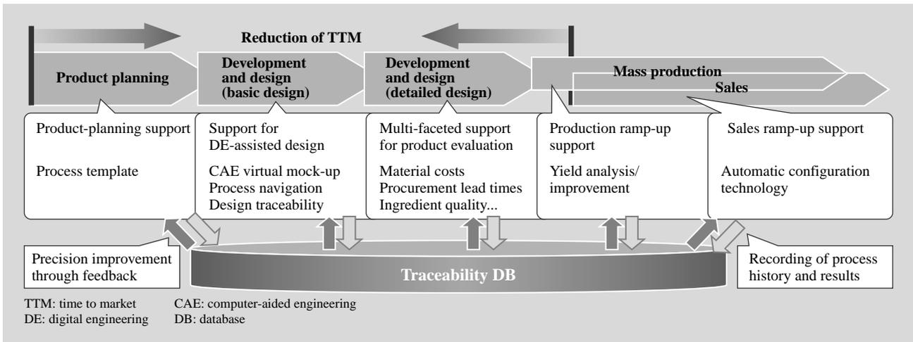
Fig. 3—Overview of Front-loading Technology for Attaining Shorter TTM. As regards the process flow for product planning, development, etc., on top of thorough specification investigation based on feedback of results, a mechanism for launching production and sales perpendicularly is necessary.
