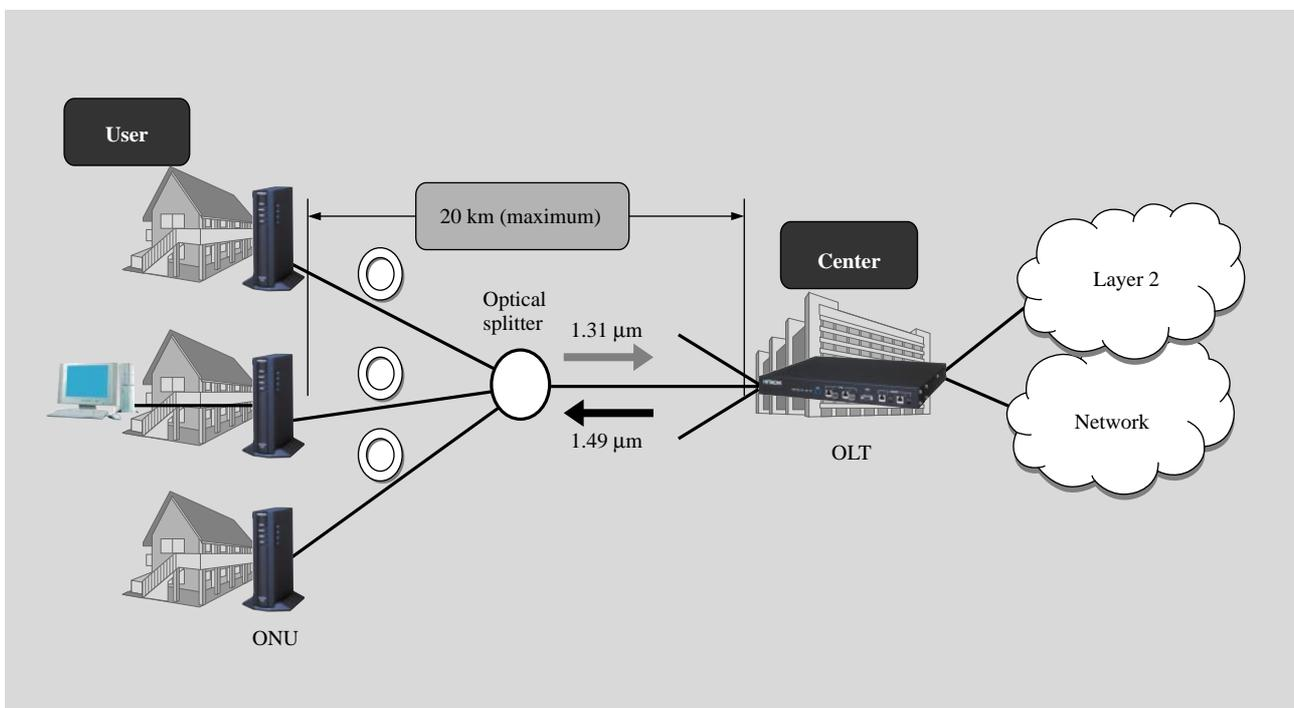
Fig. 2—Basic Configuration of Gigabit Ethernet PON.
