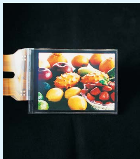
3.5-inch prototype organic EL display constructed with this technology; it is 1.8-mm thick and has 230,400 pixels (320 × 240 × RGB).
