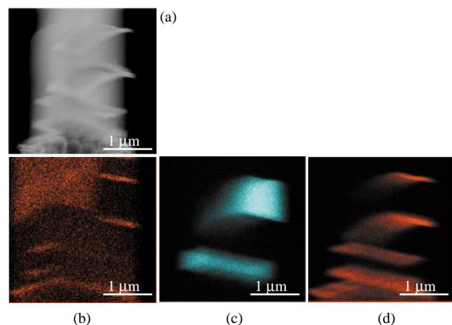
Fig. 5—Elemental Maps of Aluminum Metal Lines in DRAM (2- $\mu\text{m}$  square).
