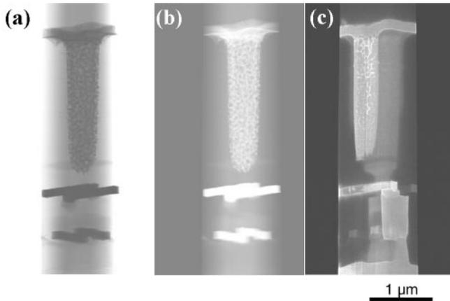
Fig. 6— (a) Bright-field Image, (b) Dark-field Image, and (c) SE Image of DRAM Capacitor Plug (size:  $0.5 \times 1 \mu\text{m}$ ). The fine structure of the insides and surface of the capacitor, interconnections, and plug can be seen in detail.
