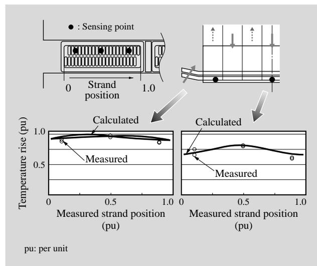
Fig. 7—Stator Core Temperature Distribution during Copper-loss Operation. Temperature homogenization in the slots was achieved.
