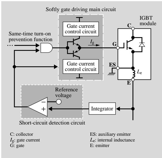
Fig. 7—System Configuration of Low-loss Low-noise Smart Main Circuit System.
