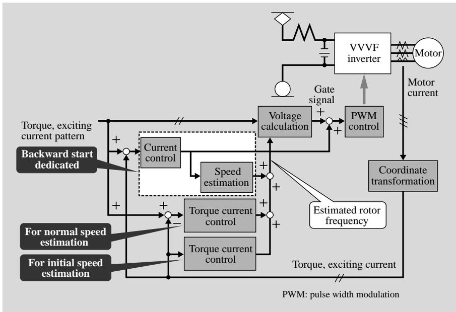
Fig. 8—Scheme for Enhancing Speed Sensorless Vector Control. Adhesion performance is improved while energy is saved, and at the same time, initial speed estimates can be obtained faster and with greater precision by adding an initial speed estimation and backward start dedicated control unit.
