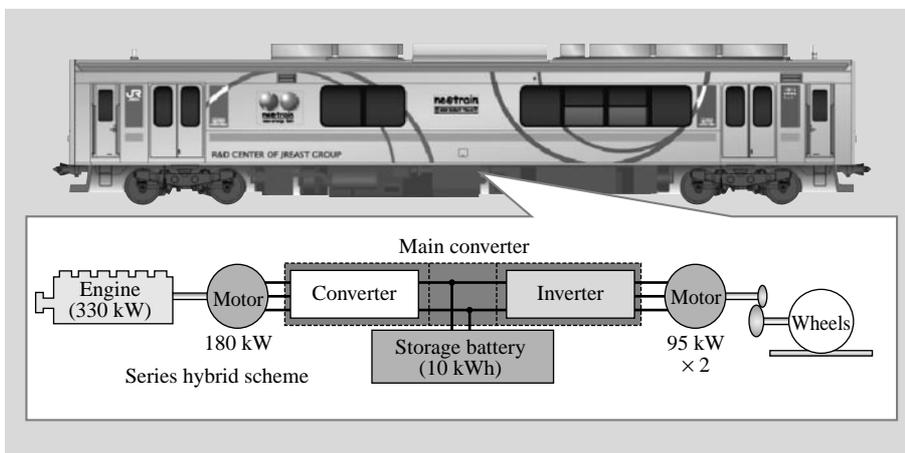
Fig. 6—Schematic Overview of Hybrid Drive System. Engine output is converted to electrical energy and a series hybrid scheme is adopted in which just the motor drives the wheels.
