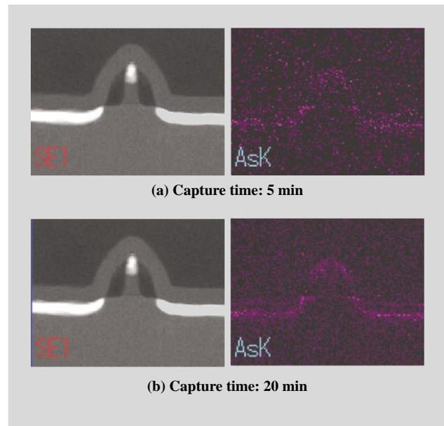
Fig. 8—Dark-field STEM Images of Si Semiconductor Device Cross-section and EDX Elemental Mapping Images. Elemental distribution images are captured 10 times faster using HD-2700 than the former system, so it should prove to be a high-throughput and highly sensitive tool for EDX analysis.
