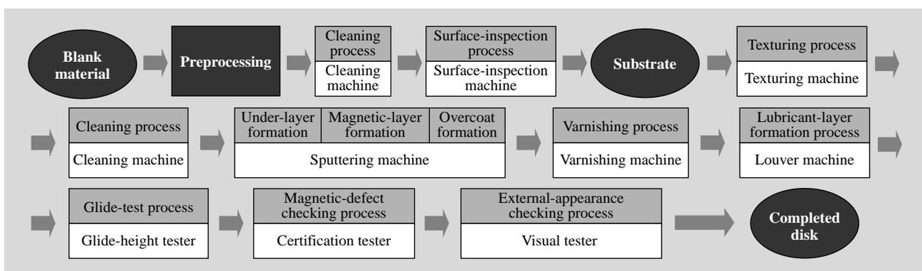
Fig. 4—Substrate and Disk-fabrication Processing.
