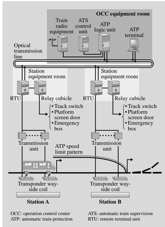
Fig. 3—Signaling System Schematic. The signaling system is supported by transponders deployed along the track, and the wayside equipment is greatly simplified by reducing equipment between stations.
