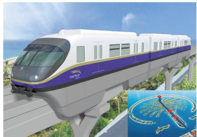
Fig. 5—The Palm Jumeirah Transit System. The project involves a driverless automatic operation system monorail connecting the Dubai mainland with The Palm Jumeirah, a new resort area on a vast artificial island. The monorail is expected to be the main access to the island.
