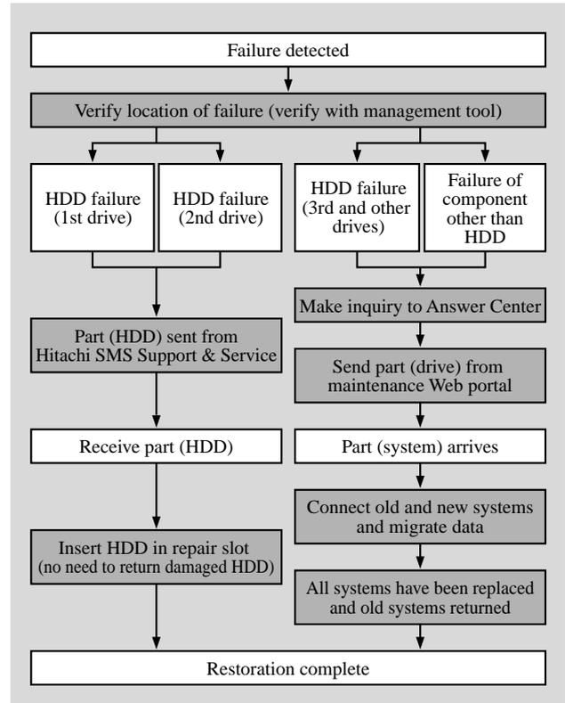
*Fig. 6—Flow for Dealing with Array System Failures. Flow for dealing with system failures in maintenance operations is shown.*
