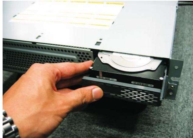
Fig. 4—Inserting an HDD into a Repair Slot.
