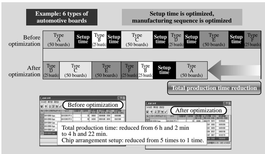
Fig. 14—Improved Productivity with the Multi-product Line Balance Software. This shows an example where the number of setup has been reduced from 5 to 1, and total production time including setup has been reduced by 30%.
