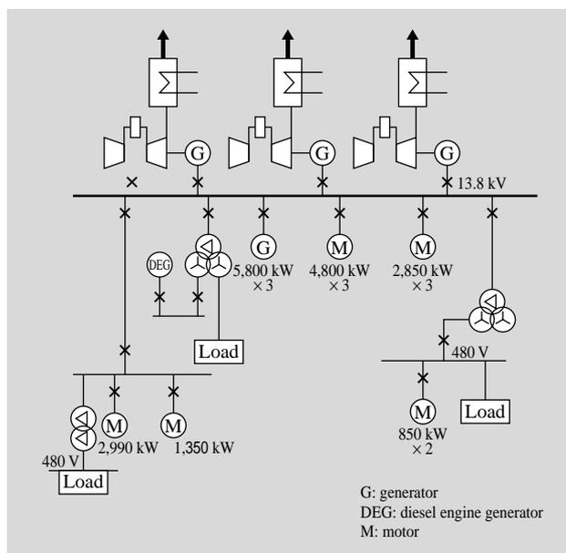
*Fig. 8—Electrical System of Betara H-25 Plant. Three H-25 gas turbines are connected to 13.8 kV line and supply electricity to the motors for gas compressors.*
