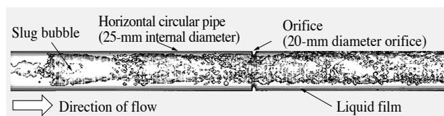
Fig. 4—A Calculated Flow Pattern of Gas-liquid Two-phase Flow in a Horizontal Pipe with an Orifice.
