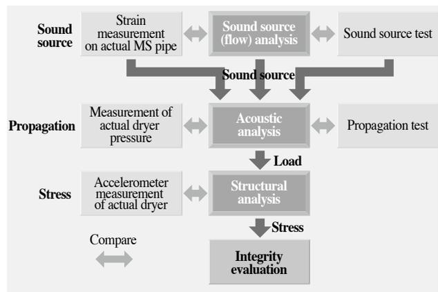
Fig. 7—Flow Chart of Acoustic Vibration Analysis of Steam Dryer. Sound source, acoustic, and structural analyses are combined to evaluate the integrity of the steam dryer.
