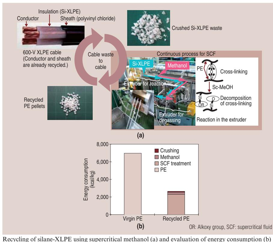
Recycling of silane-XLPE using supercritical methanol (a) and evaluation of energy consumption (b)
