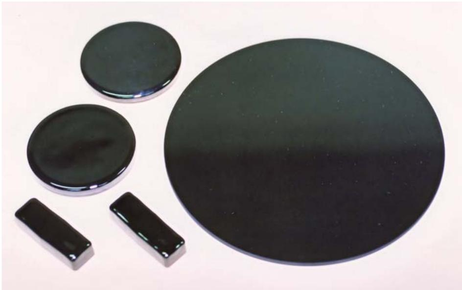
in the low-melting-point glasses used for low-temperature glass sealing and coating at 500°C or less. To reduce the burden on the environment and ensure reliability of supply, Hitachi has developed a new vanadium-based low-melting-point glass that does not use lead or bismuth.
