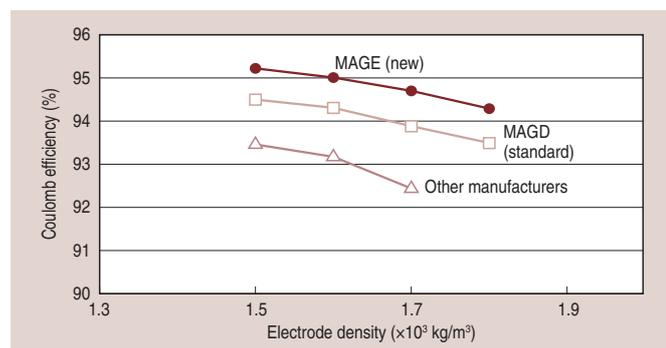
Relation between electrode density and first charge-discharge efficiency
