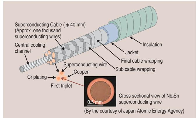
Structure of ITER TF conductor
