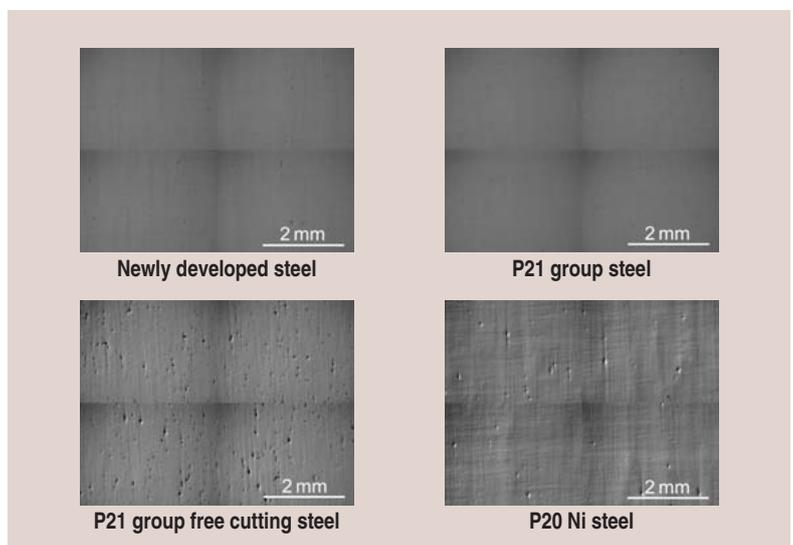
Images of specimens after #5000 mirror polishing taken using a differential interference microscope
