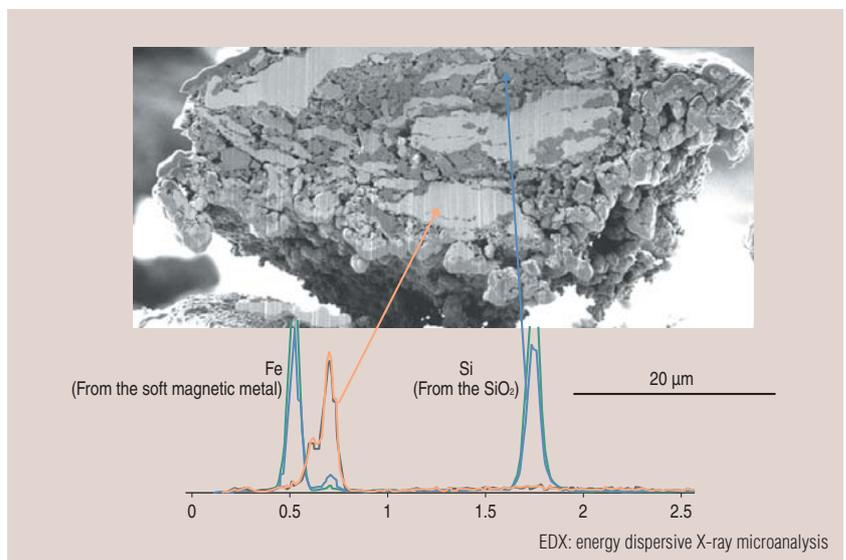
Cross section of soft magnetic metal and silica lamination structure taken using a scanning electron microscope (upper) and EDX result (lower)
